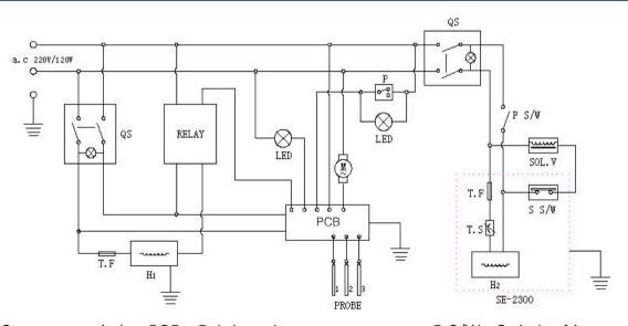
QS: power switch PCB: Pcb board
